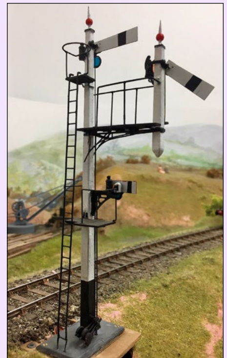
Scratchbuilt, servo operated, semaphore bracket signal with working lamps located on the station approach
